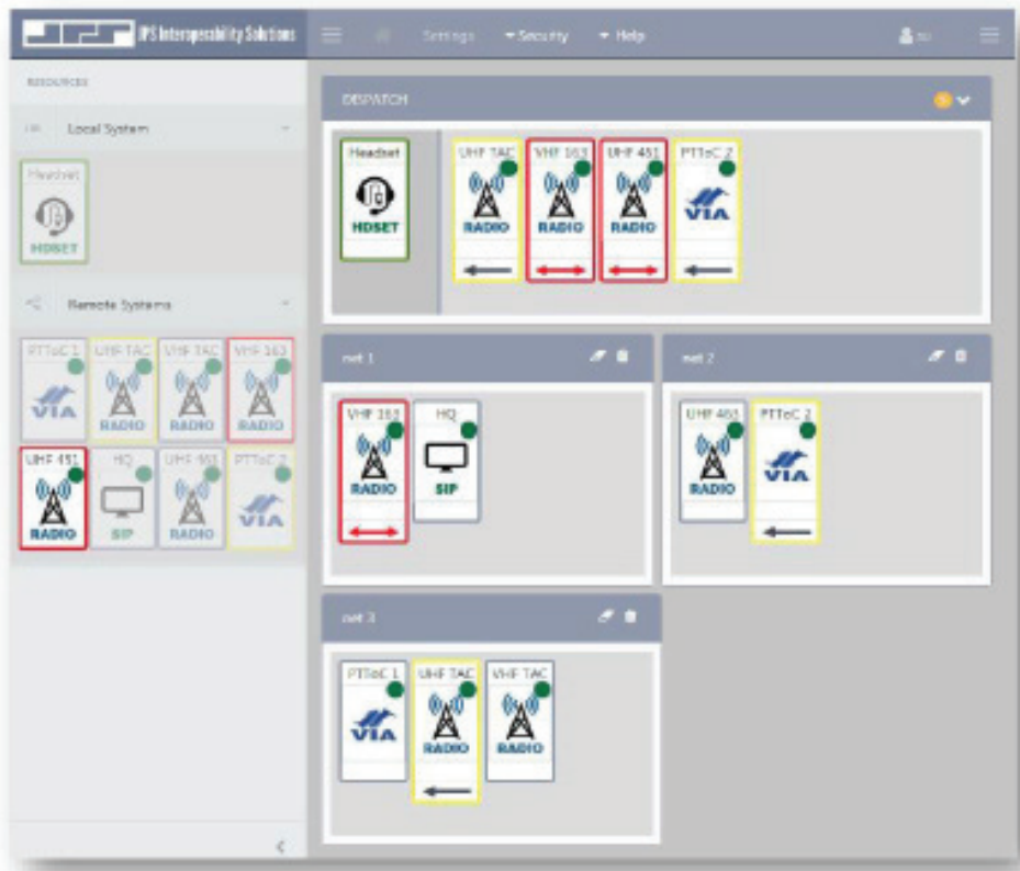
Below: The block diagram depicts a small Z2 Controller interoperability system with 8 remote voice communications channels.
