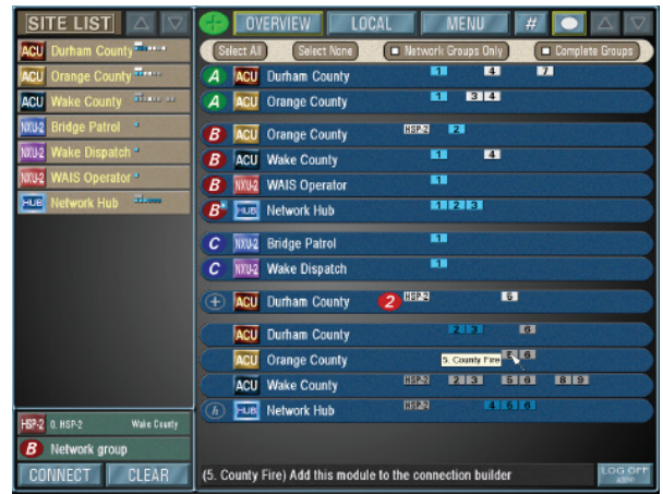
Upper: A WAIS local interoperability site featuring the ACU-2000IP radio interoperability gateway. Middle: A WAIS Controller Overview screen. Bottom: Sample WAIS block diagram.
